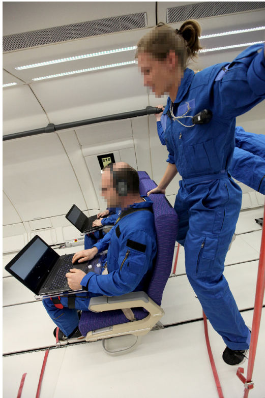
FIGURE 2 | Experimental setup in the Airbus A 310 Zero-G. Participants were buckled up in standard aircraft chairs with feet fixed to their ground floor with foot straps. The laptops were mounted to a plexiglass plate that was strapped to the participants' upper legs that allowed them to maintain the same position throughout testing. Testing was performed during 15 parabolas, providing a total of 90 trials (30 trials during 1 g, 1.8 g, and 0 g, respectively). Photo credit: Novespace/ESA.
