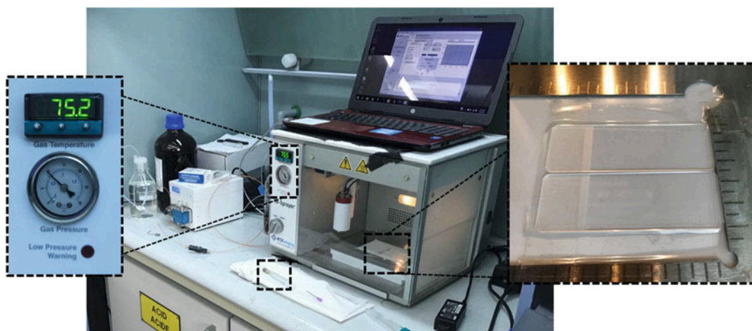
Fig. 3 Diagram of spraying apparatus. Left: Set the nozzle temperature to 75 °C and the nitrogen pressure to 10 psi. Center: Connect a syringe ( dashed box ) to the loop of the sprayer, and fill the loop with 5 mL of the matrix solution. Right: Place the samples on the plate, and begin the spraying process ( see Note 9 )
