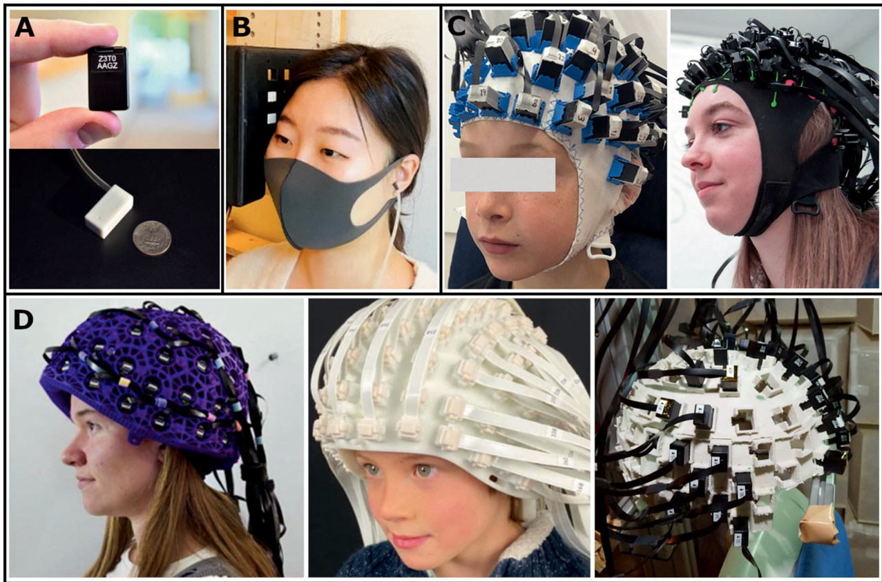
Fig. 2 OPM sensors and sensor arrays. A Size of current generations of commercially available OPM sensors is as small as a USB stick (Quspin - https://quspin.com ; Fieldline - https://fieldlineinc.com ) (B) OPM sensors can be rigidly installed around a person's head [146] (C) , onto caps, similar to EEG electrodes [25] (Quspin - https://quspin.com ) or (D) fitted into 3-D-printed helmets [147], ( https://doi.org/10.1111/nyas.14935 ). All arrangements can be adjusted for individual head sizes. No study participants are displayed in this figure and all material was edited with permission.
