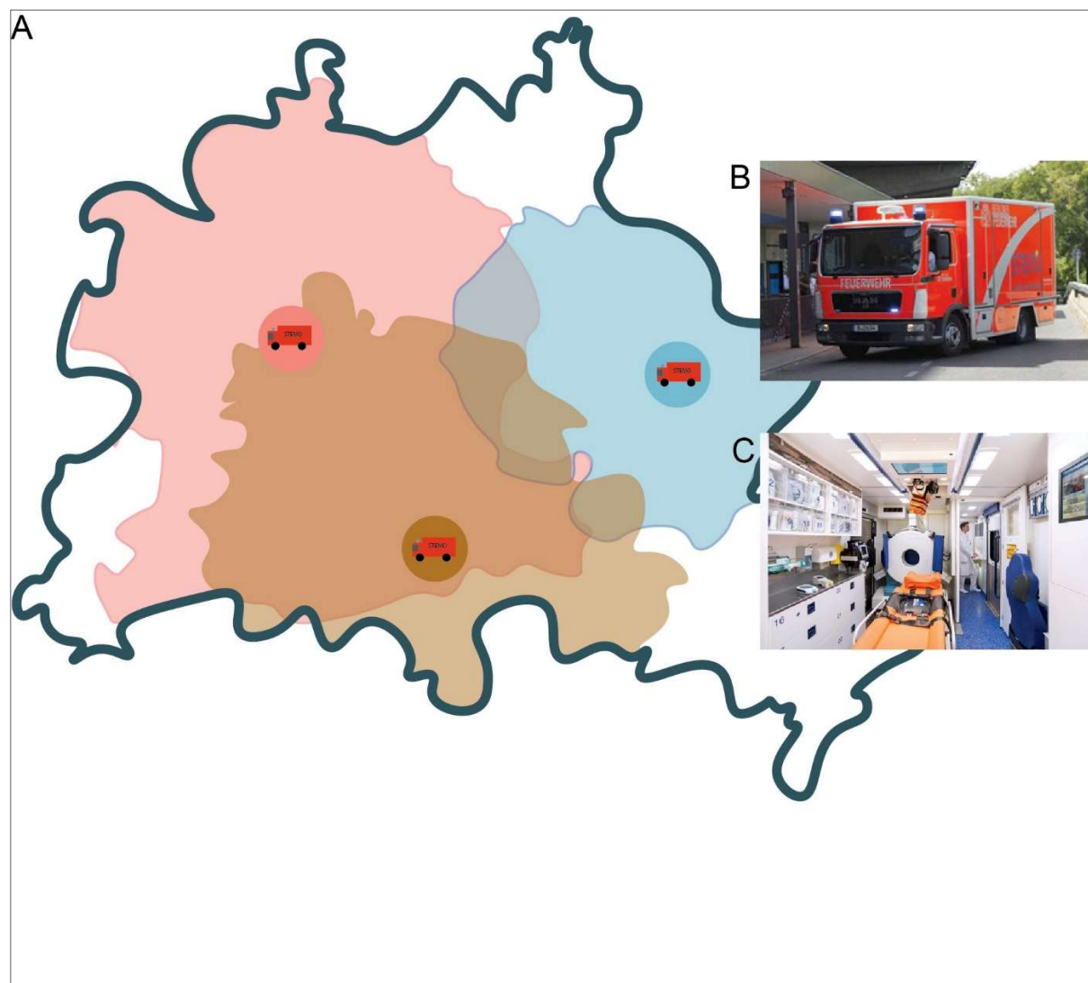
Fig. 7 (A) Catchment areas of Stroke Emergency Mobile Units (STEMOs) stationed at three locations in Berlin. Insets show the STEMO vehicle (B) mounted with a mobile CT scanner (C). Adapted from (EBINGER et al. 2021). (Images courtesy of the Berlin Fire Brigade.)
